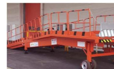
**안전난간대 (Safety handrail)**
